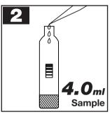
2. Pipet 4.0 ml sample into the sample vial.
